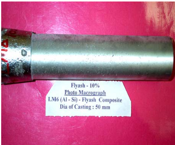
Figure 4 Photo-macrograph of Al-10% flyash MMC.
